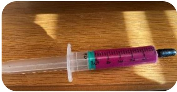
**Resources:** 5ml thermochromic paint to 1L water, 5ml syringes, water of different temperatures (no warmer than 50C), beakers or cups, thermometer.
